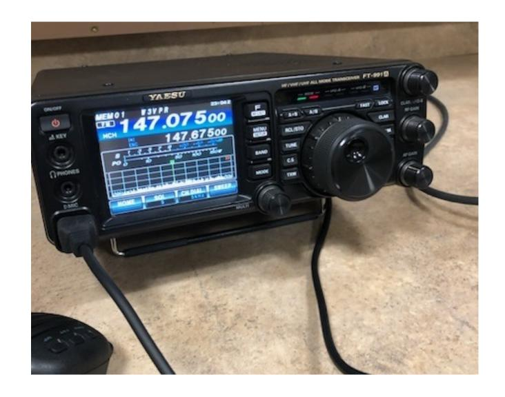
To switch from memory to VFO, push the V/M button to right of large tuning knob
