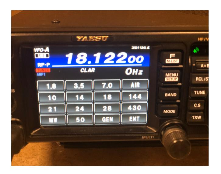
To change modes, click mode button in center of front panel, then touch desired mode
