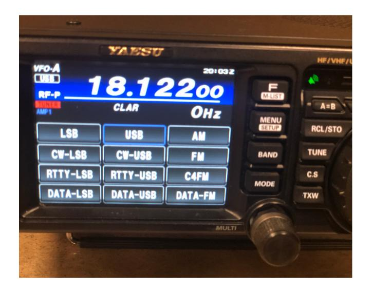
When working HF, ensure acceptable SWR before transmitting
