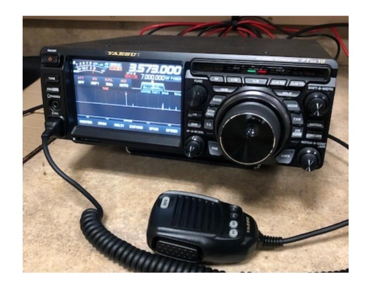
To change bands, click on the band button at 10 o'clock position from large tuning knob, then touch desired band on screen
