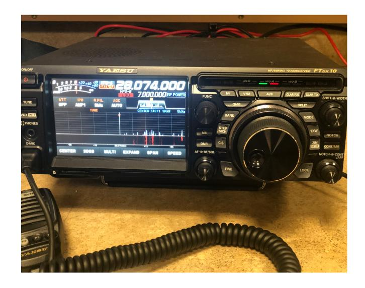
If using FT8 or other full duty cycle modes, please reduce power to 50 watts
